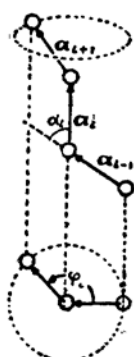
Fig. 2. Bond angle \alpha_i and rotation angle \varphi_i .
